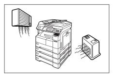
Do not install the machine near heating or an air conditioning unit.
