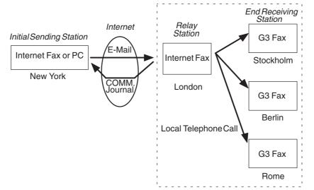
From your PC or your machine you can send documents to a Relay Station with the telephone number of the End Receiving Station(s).
