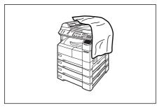
Do not place heavy objects or spill liquids on the machine.
